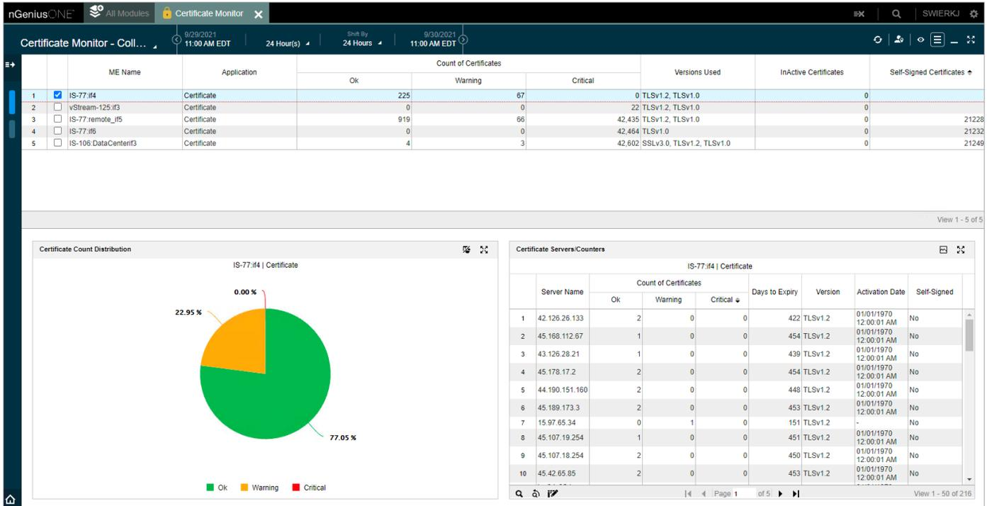
Figure 1: The Certificate Monitor view in nGeniusONE revealed details regarding SSL certificates that were approaching their expiration dates. The Security Operations team was able to proactively update the certificates and avoid an expiration.
