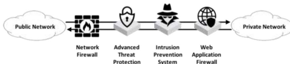
Figure 1. Inline Security Tool Deployment in the DMZ
