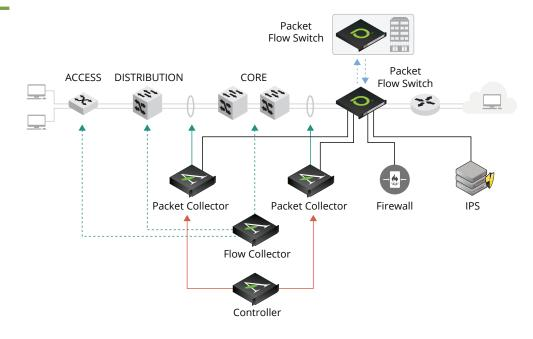
Diagram 2. NETSCOUT packet flow switches delivering to Arbor Networks packet collectors.
