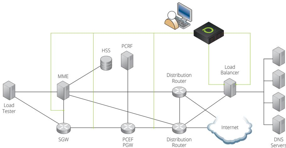
**Figure 1: Typical LTE pilot network. The customer was using a load balancing device to distribute DNS transactions across a cluster of DNS servers. The nGenius solution monitors DNS performance across the LTE/EPC and data center network tiers.**
